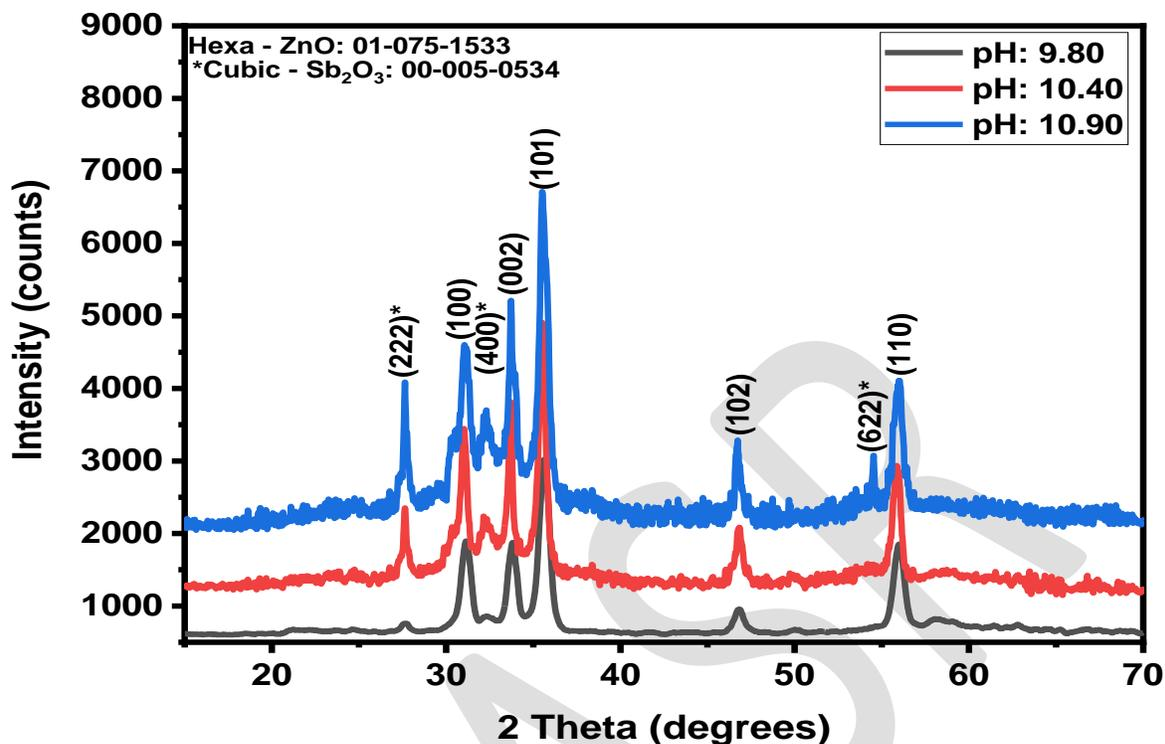
**Fig 5: X- ray diffraction pattern of antimony doped zinc oxide (Sb:ZnO) thin films formed at different pH values of 9.80, 10.40 and 10.90.**
