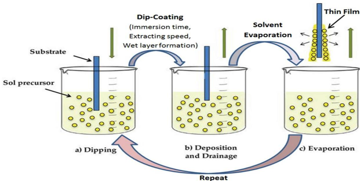
Figure 1: Schematic diagram of sol-gel deposition process (Mohamed *et al.*, 2022)
