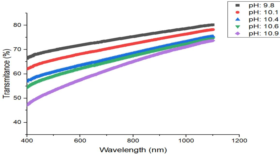
**Fig 4: Graph of transmittance against wavelength for Sb:ZnO thin film with variation in pH values.**
