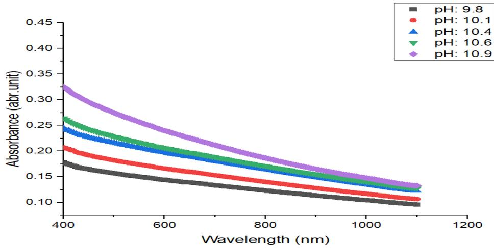
**Fig 3: Graph of absorbance against wavelength for Sb:ZnO thin film with variation in pH values.**
