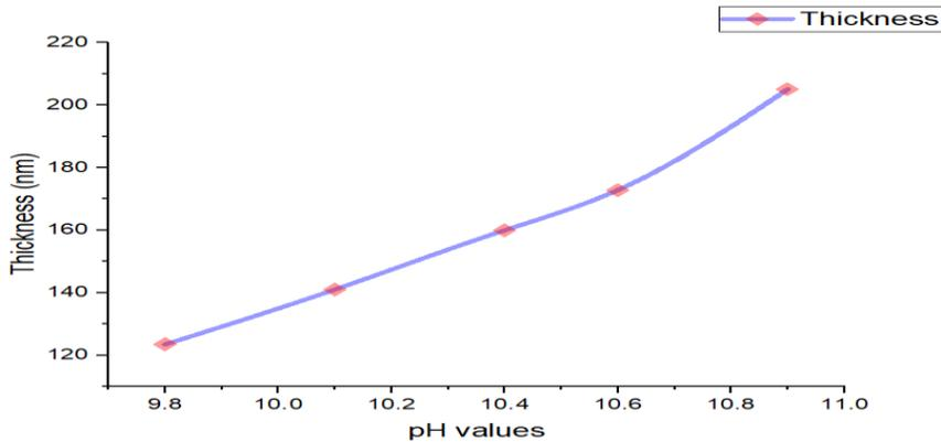
**Fig 2: Graph of film thickness versus pH values.**
